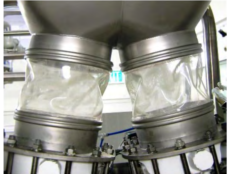
TWIN DISCHARGE TO BUTTERFLY VALVES
