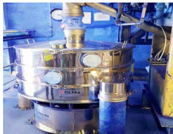
On a sifter processing paint pigment.
