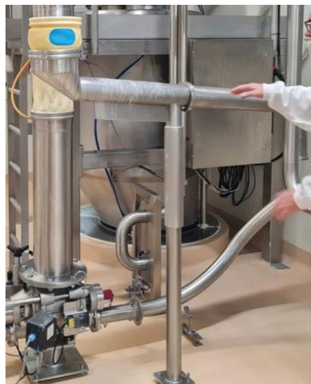
The BFM ® Corner Connector replaces expensive steel swivel tundish type setups like this.
