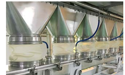
Multiple BFM's on a sifter producing MSG.
