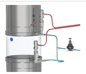
Pressurised air is pumped between the flexible cuff of the  ${\sf BFM}^{\circledast}$  connector and the spigot.
