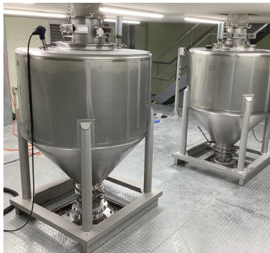
Steel buffer tank/hopper
