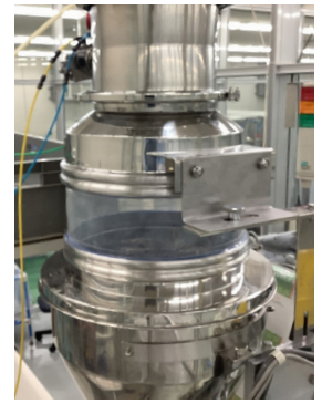
Hopper connection under Piab vacuum conveyor
