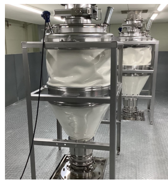
BFM® two-part hopper solution with transparent Seeflex O40E
