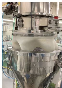
Hopper connection under Piab vacuum conveyor
