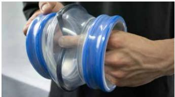
Once released, grasp the tensioner ring with your fingers and pull the entire ring out of the connector completely.
