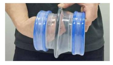
From the outside, apply force to push the tensioner ring inwards to release it from the formed portion of the connector.
