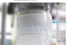
When inflated, the outer Seeflex layer will securely hold the bag neck up and open for clean, efficient filling.
